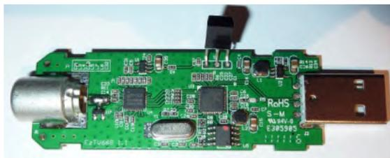
Freq response for Elonics E4000 device is 64MHz to 1700MHz. No good for HF, or even SSB, but a very cheap way to get into SDR and to learn what it has to offer.
