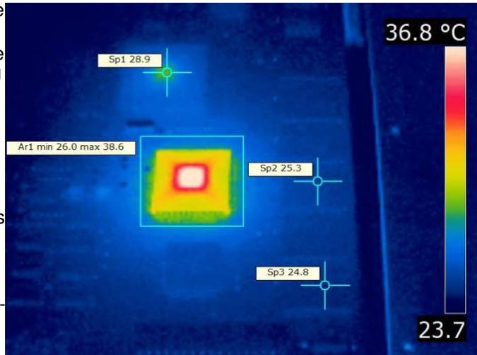
The #1 IHU showed some abnormal heating of one of the 6 memory chips on the right side of the photo below. With the Infra red thermography, temperatures are relative and although the two large chips look
