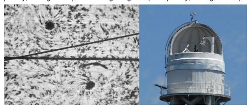
Remember that swirling action that Hale noted? Well, looking at the <u>magnetogram</u> of a given sunspot, you see either the bright spot leading or trailing the group versus solar rotation, and this flips when the Sun's poles reverse every solar cycle.
